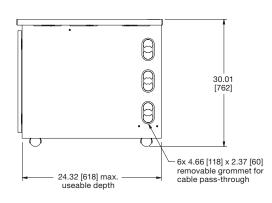
LD-1230\_\* side rack gangs to desk w/ included hardware and provides 12 rackspaces for equipment mounting behind an attractive smoked plexi front door. In order to join LD-1230\_\* side rack to LD wedges, the LD-WK joiner kit is required.
